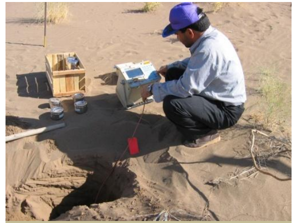
Figure 3: Measuring soil moisture by time domain reflectometry (TDR)
